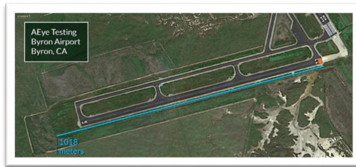
Figure 1: Bird's eye image of Byron runway 5/23 with blue line representing the length of the runway, the distance driven in reverse by the AEye research vehicle (with mounted iDAR sensor). The orange dot represents the Chevy Bolt and Mercedes-Benz Sprinter delivery van.
