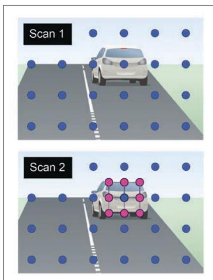
Figure 3. Packing a dense 3 x 3 grid around a detect allows the collection of more useful data and greatly speeds up classification. Scan 1 above has a single detect on a vehicle. Rather than wait for the next frame to resample this vehicle (as is the traditional mode in LiDAR) we instead quickly form a dedicated dense ROI, as indicated in Scan 2 below. This is done almost immediately after the initial single detect and before completing the next scan.
