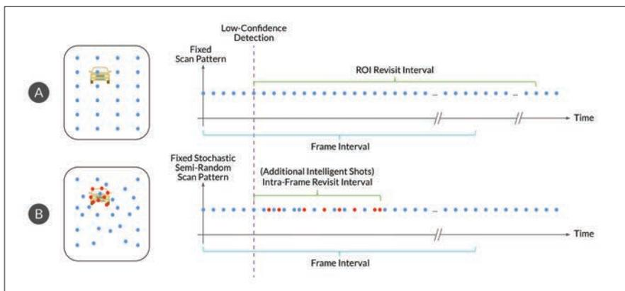
Figure 1. Advanced agile LiDAR sensors enable intelligent scan patterns such as the “foveation in time” intra-frame revisit interval and random scan pattern of the AEye solution (B) compared to revisit interval on a typical fixed pattern LiDAR (A).
