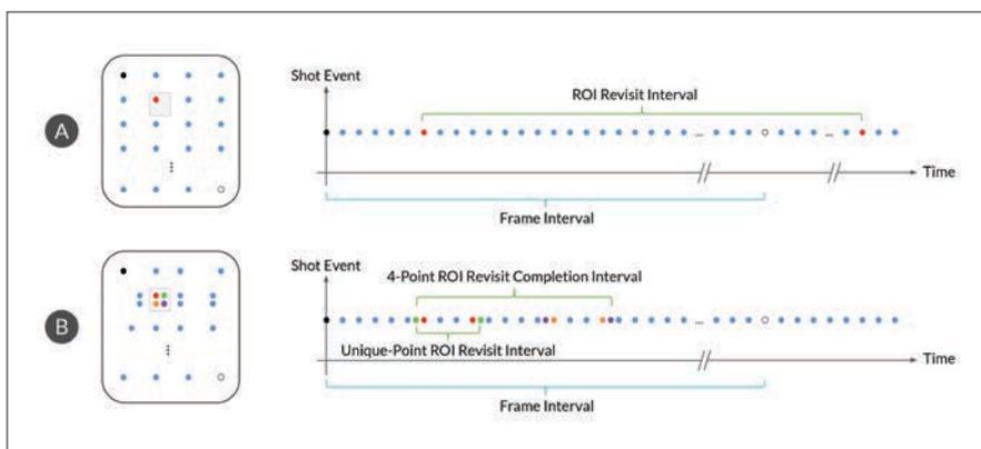
Figure 2. Region of interest (ROI) revisit rate and foveation of the AEye solution (B) compared to conventional scan patterns (A).
